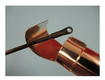
Push the tail pushrod into the pushrod holders D59, push the ball joint on the ball of the tailservo arm and adjust the arm rectangular. Attach a ball joint 041 on the bellcrank D49 and adjust the bellcrank also rectangular following the inner contour of the bellcrank.Now place a mark with a thin felt marker about 1mm before the end of the ball joint and remove the pushrod again.
