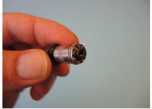
Then add the blue marked grooved shim with the inner diameter 5.0mm (does not tilt). The outside should correspond with the end of the tailrotor hub D255.
