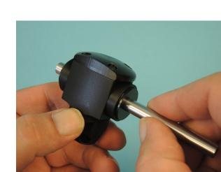
Add a washer shim 8x14x0.5 047, a ball bearing 8x16x5 071 and a threaded bush 509.
