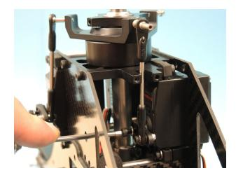
The cable of the tailservo is pushed into the left slot of the gyro plate D621. Therefore it is eventually necessary to remove the front threaded block D23a.
