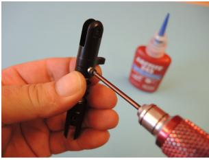
View of the mounted unit. Both blade grips should turn easily and a small end play is recommended to keep both thrust bearing without any load. If this is not the case then disassemble the unit and shorten the conic bushes a bit using a file or sandpaper. If the endplay is too much then use a 0.1mm washer shim that you place between inner bearing and blade grip mount ring.
