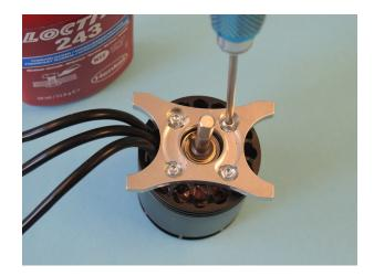
Push the motor pinion D37 (18-22 teeth) on the shaft so that one threaded hole is corresponding with the flat spot on the motor shaft. Check for a clearance between pinion and motorplate of 0.5-1mm. Then tighten the pinion on the flat spot with a grub screw M4x5 035 using Loctite. Add then a second grub screw M4x5 035 using Loctite and tighten it.
