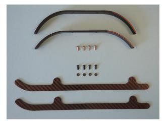
Parts overview of the landing gear with aluminum skids (alternatively).
