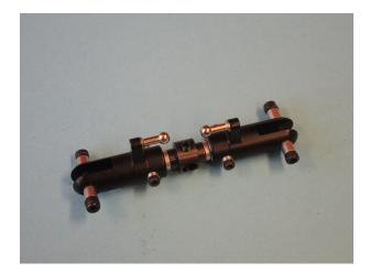
Fully attach two shortened ball joints 385 on the threads of the knuckle joints 382 of the tailslider 1475. They should be positioned so that the numbers on the ball joint should show like placed in the picture on the upper joint to the left side and on the lower to the right.
