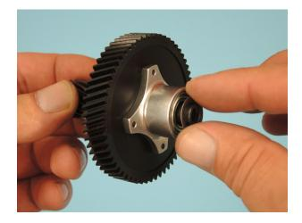
Push the lower bearing block D612 with the flanged bearing D70 onto the shaft showing with the flanged side of the ball bearing to the freewheel unit. Note the different inner contour of the bearing block. The rounded side is the longer side that is on the left side (view in flight direction).
