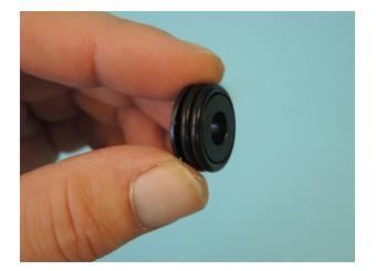
... and press these units in teh main rotor hub D52. We do not recommend to lubricat6e the O-rings. If you do it please use only a very bit of lubrication on the outside of the O-rings.
