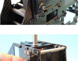
Now press the cutted rubber grommet into the hole as long as it snaps. If the grommet is going thru the hole during pressing then remove it from the servo cables, put it on them on the other side and try again.
