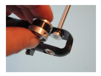
Bend the staple in that way that it can be used for pulling the rubber ring D66 thru the bush D60. Place the two ends of the rubber ring into the staple...
