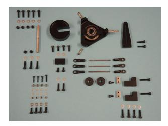
Attach two joint bolts M3x9 078 with rich Loctite on the two free arms of the swash plate D630. The swash plate guide D530 is already factory mounted with Loctite.
