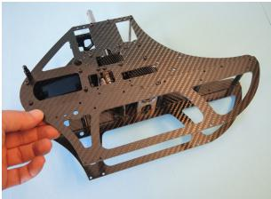
Add at the rear end (as on the left side too) a hex bolt M3x8 D197 and a lock nut M3 008s and tighten it.
