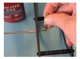
Attach the conroller platform D42 with four countersunk screws M3x8 025. Therefore place the holes in the connectors vertical. The mounting wire can help to find the vertical position.
