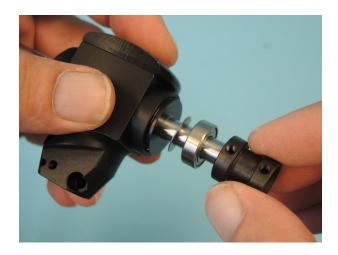
Add the thrust bearing 8x16x5 100. First add the non marked grooved shim with the inner diameter of 8.2mm (tilts on the spindle). Press a bit of lubrication in the groove.
