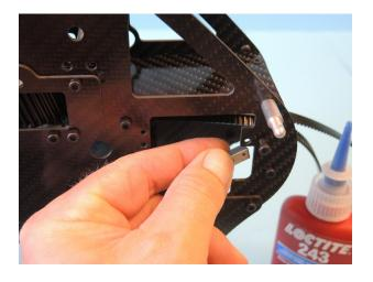
The roll servo is attached with four hex bolts M3x12 D119, washers M3 002 and lock nuts M3 008s. Therefore the open wrench #707 is a very good tool. The lower right screw will be applied with Loctite and turned then in the connector D622. After gently tightenimng of the bolts the provisorically mounted single bolt on the right side can be removed.
