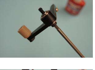
Push the threaded end into the pushrod so that about 7-8mm free end should be out. Remove the unnecessary resin careful.
