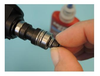
Add two lens screws M3x6 D199 using Loctite. Before tightening push both bladegrips in outside direction to eliminate play between screws and crossholes of the bladegrips.
