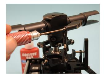
Attach the double ball joint linkage with a lense screw M3x12 989 and enough Loctite on the swashplate.
