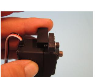
Attach the elevator servo from inside into the hole of the upper right side frame D602.
