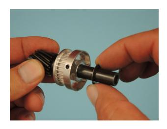
Push the mounted freewheel unit on the pinion shaft D609.
