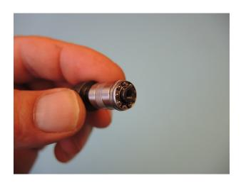
Then add the blue marked grooved shim with the inner diameter 5.0mm (does not tilt). The outside should correspond with the end of the tailrotor hub D255.
