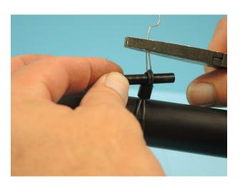
Position the pushrod guides in that way on the tailboom that each free distance is about the same (tailservoarm/guide/guide/tail bellcrank).
