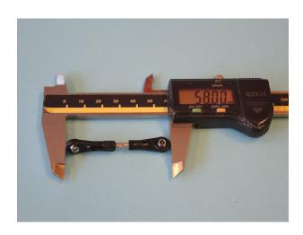
Attach the double ball joint linkage with a lense screw M3x12 989 and enough Loctite on the long blade grip arm.
