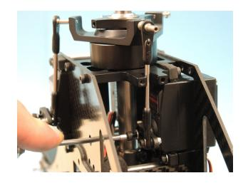
Attach the swash plate holder D532 with two hex bolts M3x12 D119 using Loctite.
