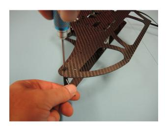
Then add a hex bolt M3x8 D197 at the rear end and tighten it with a lock nut M3 008s.
