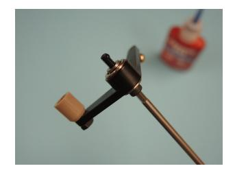
... and mount the bellcrank on the rudder fin holder D49. Note that the ball of the tailslider 1475 must be pushed into the ball guilde bush D288.
