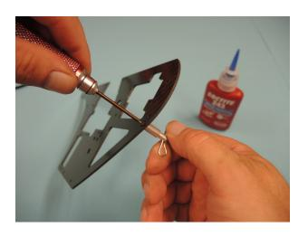
Now place the upper right frame D601 on the unit and check all holes for correct corresponding.
