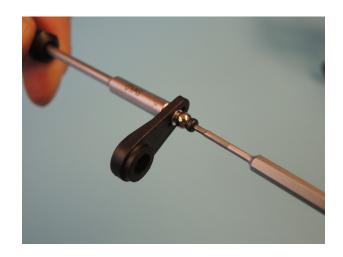
Push a rubber grommet D80 that is cutted from one side on the elevator servo cable, put the plug into the hole of the upper right frame D602 and press the grommet into the hole.
