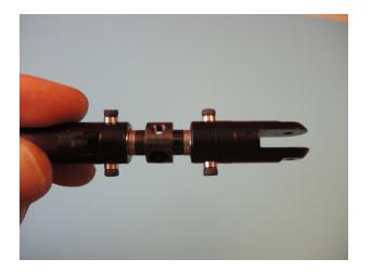
Attach a joint bolt M3x9 078 into each blade grip using Loctite. Recommended torque 1.1 Nm.
