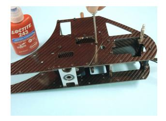
Connect the cover plate with the first stage bearings blocks D612 and D613 using four hex bolts M3x6 D196 and Loctite. Keep them still loose.
