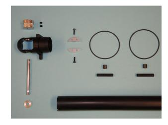
Remove some anodized black surface from the front end of the tailboom D639 (the side without slots) with a small flat file to get a good grounding between tail and mainframe. For this reason the front tailboom clamp is not anodized. Then push the tailboom careful in the clamps. Be cautious that you do not damage any servo cable.
