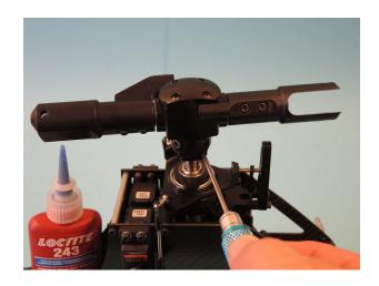
Push on the SRC arm D545 the spacer bush D637 and mount a ball joint M3 D72. If necessary add washer shims 3x6x0.1 475 between spacer bush and ball joint so that the ball joint has a tight contact and is to the same time positioned rectangular.
