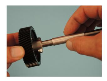
Push the upper main shaft bearing plate D607 on the mainshaft. The flange of the ball bearing D71a must show to the spacer bush.
