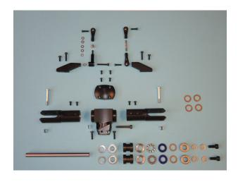
Thr mainrotor hub cap 580 ist attached on the mainrotor hub D452 with four lense screws M3x6 D199. The spindle bushes D453 are already factory attached.
