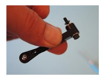
Mount the SRC arm on the shorter blade grip arm D636 with enough Loctite. Be careful beneath a ball bearing using Loctite. Capillar forces can pull too much applied Loctite into the bearing.
