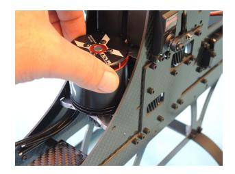
Mount the motor carrier D633 with four hex bolts M3x8 D197 and washers M3 002 using Loctite.
