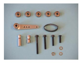
Two ball bearings 3x10x4 064 are pushed on a lense screw M3x12 982, followed from a washer shim 3x6x1 051 and will be attached with Loctite on the belt tightening lever D614.
