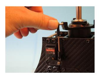
The roll servo arms and the elevator servo arm are attached with a hex bolt M3x8 D197 and a washer shim 3x6x1 051 using Loctite. This step should be done later when electric current is on the servos and they have their real center position.
