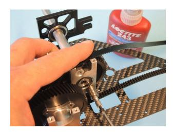
The premounted belt tightening lever will be screwed with Loctite into the left hole of the lower mast bearing block (seen in flight direction). Please check before that the washer shim 3x6x0.2 455 is placed between the upper bearing of the lever and the lower mast bearing block. After tightening check the lever for easy turning.
