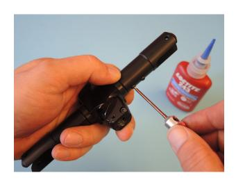
Add on the blade grip arms a hex bolt M3x8 D197 and a hex bolt M3x14 D198 and apply Loctite on the threads.
