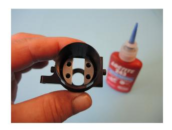
Push the tailrotor housing fully on the boom and check, looking inside, that the boom has really mechnical contact to the end of the housing. Check also that the brackets are vertical in the boom. Then tighten the bracket screws.
