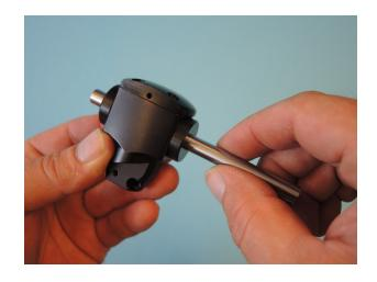
Add a washer shim 8x14x0.5 047, a ball bearing 8x16x5 071 and a threaded bush 509.
