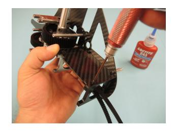
Put the vertical frame stiffener D623 into the slot of the right frame and check for clearness, eventually file the edges a bit. Check the same on the slot of the upper rear frame D601.
