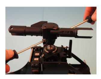
Tighten the two hex bolts M3x12 D119 in the mainrotor hub.
