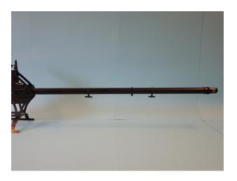
Attach the rudder fin D640 on the rudder fin holder D44 with two hex bolts M3x8 D197 using Loctite.
