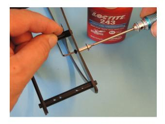
Attach the right front canopy holder D619 on the same way with a lense screw M3x10 989.
