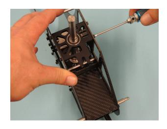
Check the gear mesh again and if necessarry follow the procedure of the assembly of bag 2. The mechanic should now stay on the ground without any tilting. If not, loose srews again and retighten them.
