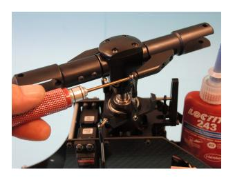
Attach the double ball joint linkage with a lense screw M3x12 989 and enough Loctite on the swashplate.
