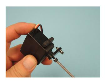
Two tail servo mounting blocks D629 are attached gently with four hex bolts M3x12 D119 and washers M3 002 using Loctite. The rubber grommets of the servo should be in straight position after tightening the screws.
