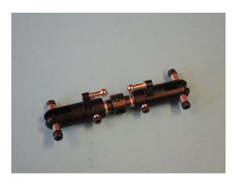
Fully attach two shortened ball joints 385 on the threads of the knuckle joints 382 of the tailslider 1475. They should be positioned so that the numbers on the ball joint should show like placed in the picture on the upper joint to the left side and on the lower to the right.
