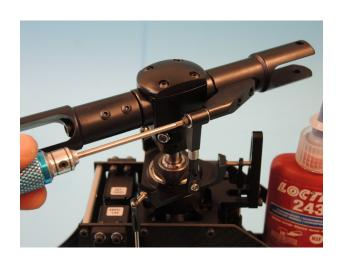
Attach the SRC arm with a lense screw M3x12 989 on the swashplate with enough Loctite.
