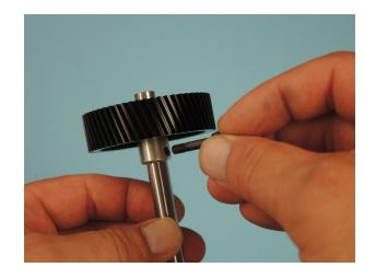
Push the spacer bush D606 on the shaft.
