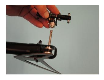
Adjust the tailrotor on the shaft in that way that the threaded M4 hole of the tailrotor-hub is corresponding with the flat spot on the tailrotorshaft. Tighten now the unit with a grub screw M4x5 035 using enough Loctite.
