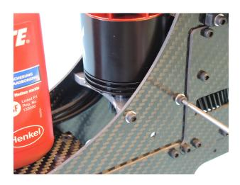
Check the gear mesh. If you move the delrin wheel slightly in both directions you must feel a small play between the gear wheels. If the mesh is too small or too large then open the motor plate mounting screws again and move the motor a little bit. Then tighten the screws again.
