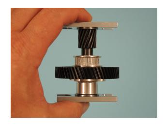
Add the toothed belt 713 in the belt wheel and position the unit as shown on the corresponding holes of the frame.
