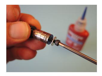
For tightening put in a wrench or a shaft into the center bore of the hub. Recommended torque is 1.5Nm.
