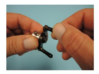
The bellcrank D49 is attached with a ball guide bush D288 and a special lense screw 092 using Loctite.
