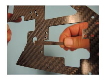
Break the edges of the cable slots in the gyro platform careful with a small needle file.
