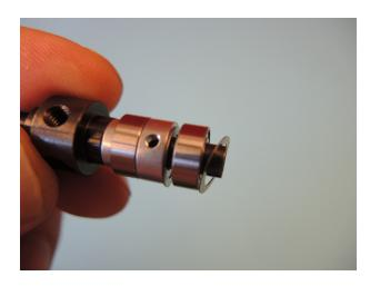
Add the thrust bearing 5x10x4 112. Begin with the non marked grooved shim with the inner diameter 5.2mm (tilts) and add in the groove a bit of lubrication.
