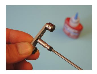
A hex bolt M3x30 D337 is pushed into the shorter dampening rubber holder (longer end of the holder outside).
