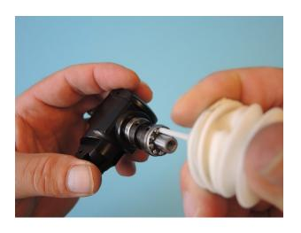
Finally add the blue marked grooved shim with the inner diameter of 8.0mm (does not tilt on the spindle).
