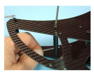
Attach the lower right frame D625 and check all holes for corresponding.
