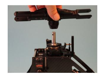
Push the jesus bolt D78 thru the corresponding holes of mainrotorhub and mainrotor shaft and tighten it with a lock nut M4 009. If the bolt cannot be easily mounted then turn the head 180 degree on the shaft and try again.
