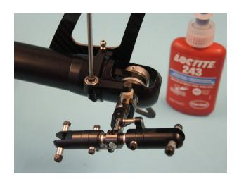
For mounting the threaded ends 087 on the tail pushrod 0350 mix some JB Weld.
