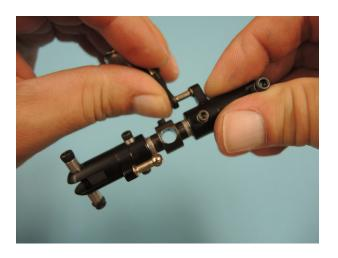
If the ball joint is too tight then press gently with a blunt pliers on the outside of the (mounted) ball joint as long as it is free enough. Do this step careful in small steps. If you press too much in one step you could get play on the joint that is not more to elimante.
