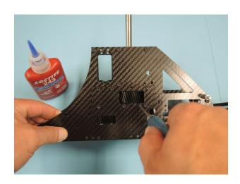
Now press the complete frame on a flat surface and tighten all screws on both frame sides (except the two lower right tail boom clamp screws).+---+
