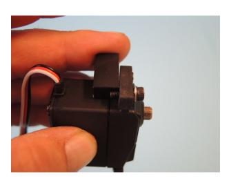
Mount the spacer block now gently on the servo cable side with the fitting screws. The screws should be not too loose and not too tight.
