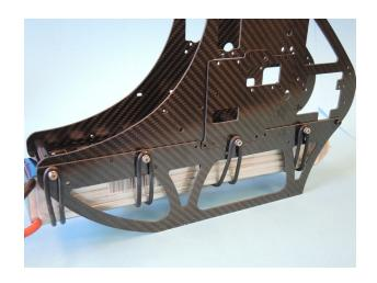
The third O-ring mounting point is attached on the left side with a O-ring holder D57 and a hex bolt M3x14 D85 using Loctite. For the connection on the right side as shown in the picture a hex bolt M3x16 D86, a O-ring holder D57 and a spacer bush 2mm D79 using Loctite are attached.
