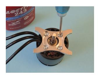
Push the motor pinion D37 (18-22 teeth) on the shaft so that one threaded hole is corresponding with the flat spot on the motor shaft. Check for a clearance between pinion and motorplate of 0.5-1mm. Then tighten the pinion on the flat spot with a grub screw M4x5 035 using Loctite. Add then a second grub screw M4x5 035 using Loctite and tighten it.
