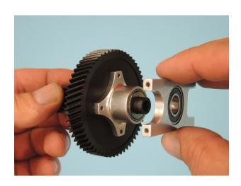
Push the upper bearing block D613 (with the cover plate) and the flanged bearing D70 onto the upper pin of the pinion shaft showing the flange of the bearing to the toothed gear wheel.
