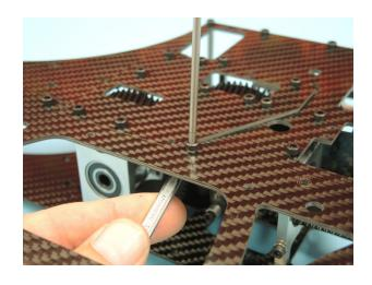
... and also this shown point will be connected with a hex bolt M3x8 D197 and a lock nut M3 008s. Attach the delrin connectors D626 after that to make the tightening of the screws easy.
