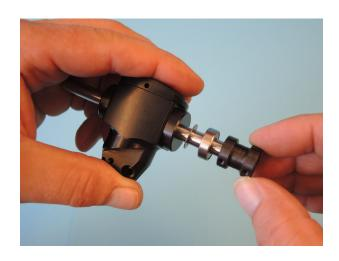
Add the thrust bearing 8x16x5 100. First add the non marked grooved shim with the inner diameter of 8.2mm (tilts on the spindle). Press a bit of lubrication in the groove.
