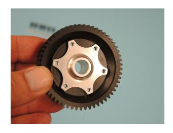
Add six washers M3 002 to six screws M3x8 D197 and apply Loctite on the threads.
