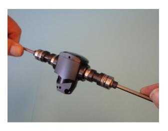
Attach two hex bolts M3x12 D119 in the rotorhub D452 using Loctite.
