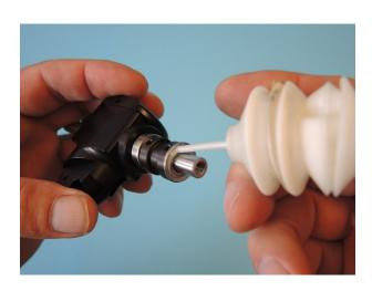
Add the ball cage as shown and add a bit of lubrication on the balls.
