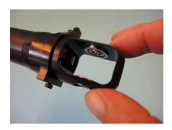
Push the tailboom as far as possible in the mechanics so that the tailbelt is as long as possible out of the tail housing. Then place the tail belt wheel 20T D643 in the belt end in that way that the mounting threads are on the left side (seen in flight direction).
