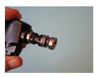
If the end play is correct then apply Loctite to the threads of both hex bolts M5x12 034 and tighten them from hand first.
