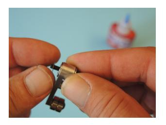
The fixed roller is now screwed with Loctite into the right hole of the lower mast bearing block (seen in flight direction). After tightening the screw all bearings will be checked for clearness.
