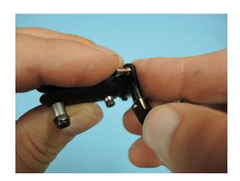
Push now tailslider and tailrotor onto the shaft that the outer end of the tailrotor hub corresponds with the end of the tailrotorshaft. The tailslider should move free. If the tailrotor is difficult to push on the shaft then turn it 180 degree using the other side of the center bore.
