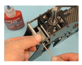
Add the cover plate D603 and check for corresponding holes.
