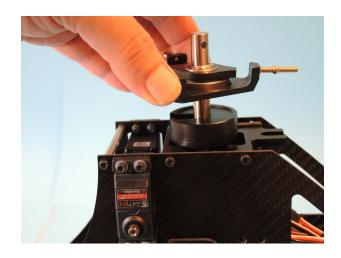
The 4mm hole in the upper left side frame is thought for (later) mounting the servo arm on the elavator servo.
