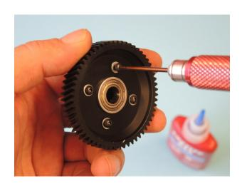
Push the belt wheel D610 on the pinion shaft D609 upto the end. First add now a grub screw M4x5 035 with Loctite on the area of the shaft with the flat spot and tighten it. Then add a second grub screw M4x5 035 in the second threaded hole with Loctite and tighten it. Finally add a washer shim 10x16x0,2 033.
