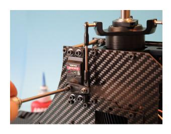
Attach the elevator servo linkage as shown. Mount the servo arm hex bolt M3x8 D197 and the washer shim 3x6x1 051 using Loctite also later when the servo is under electric current and has its defined center position.
