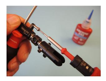
The tailrotor blades will be hold from a hex bolt M3x25 D336, two chinese weights 952 and a lock nut M3 008s.
