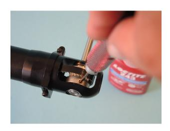
Now tighten the tailbelt. Push the tailboom out of the clamps as long as the belt tighening lever will get about the position shown in then picture. Then adjust the tailrotor shaft rectangular to the mainrotor shaft and tighten the two long hex bolts M3x35 D338 in the tailboom holder clamps using Loctite. Check that the 3mm thick spacers bushes D620a are under the bolt heads. After that tighten the two remaining lower right hex bolts M3x6 D196 of the tailboom clamps using also Loctite.
