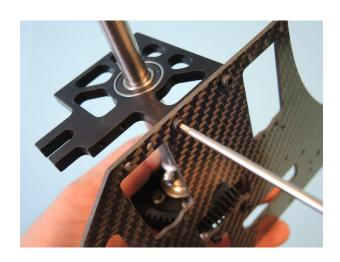
After tightening the four screws check the mainshaft for easily turning without any endplay.
