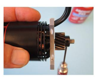
Push the motor unit between the frames so that the motor cables are placed on the right side (seen in flight direction).
