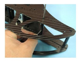
Attach the left canopy holder D619 with a lense screw M3x10 989. Use no Loctite here.
