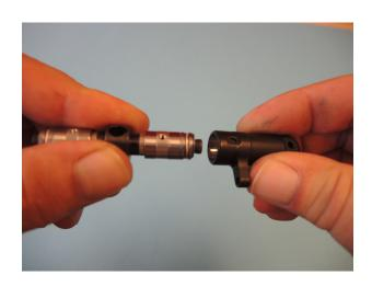
Each blade grip is now fixed with two hex bolts M2,5x5 and distance bushes 988 using Loctite. Before tightening them pull the blade grips outside so that both are corresponding with the screws.
