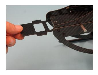
Push the battery pin in from the left side. Check the right position of the battery plate as long as the pin fits into the eyelets D456.
