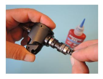
Then tighten the screws with 8-10 Nm about (if you have a torque driver). If not then "tighten, but no too tightened"). Note that a too high tightened bolt reduces the total strengthness of the bolt that can cause a damage.
