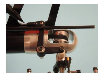
Cut the tail pushrod with a Dremel or a similar fast turning tool and attach now the second threaded end in the pushrod on the same way.
