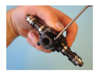
Push the bladegrips D635 on so that the cross holes in the grips are corresponding with the holes of the threaded bush 509. The fitting of the grips is quite narrow. A light warming up of the grips with a hairdryer does help.
