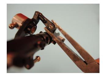
Now add the second ball joint on the other (!) joint bolt and remove then (to avoid changing) the first ball joint from the ball. Do the same procedure again. It is important that both pairs must be kept as pairs and should not be changed.
