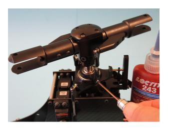
The right/left threaded linkage is made from the right/left threaded pushrod D541, a ball joint M3 D72 and a shortened ball joint M3 D578. The shortened ball joint is placed on the side with the rightturning thread (cw, no thin groove on this side).
