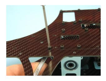
Add the remaining four delrin connectors D626 with four hex bolts M3x10 D328. It is recommended to tighten the connectors at this point only as far as they can be still turned a little bit. So the later mount of controller and battery plate will be easier.
