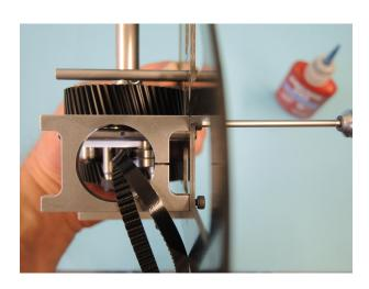
The rear tailboom holder clamp D620s is attached with two hex bolts M3x6 D196. Here the upper bolt will be tightened with Loctite too and the lower bolt is still kept loose without Loctite.
