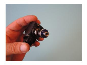
Add (a) washer shim(s) and a ball bearing 8x16x5 071. The necessary thickness of washer shims can vary a bit and must be checked by everyone for himself. Therefore both sides of maingrip units must be mounted and the M5x12 hex bolts 034 and washer shims 5x10x1 052 will be mounted from hand(!). If you feel end play then add 0.1mm on each side. If the bearings become notchy then remove 0.1mm each. You can also mount 0.1mm only on one side if necessary.
