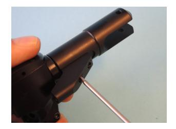
Attach the rotorhead on the mainshaft. The tolerance of the bore is narrow tolerated. During pushing on tilt the head slightly in both directions. Also a drop of oil is helpful. Do never turn the hub onto the shaft (risk of seizing)!
