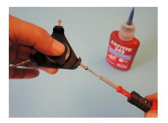
Attach two threaded blocks D23a with two hex bolts M3x8 using Loctite at the tail-servo cut-out of the upper left side frame D601. Add for perfect corresponding holes a second screw in the block before you tighten the first one. After tightening remove the second one.
