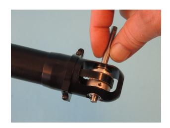
Add a grub screw M4x5 035 using Loctite in the belt wheel thread that is corresponding with the flat spot of the tailrotor shaft. Check that the left end of the shaft is corresponding with the outside end of the ball bearing. After tightening this screw add another screw M4x5 035 in the belt wheel using Loctite and tighten it.
