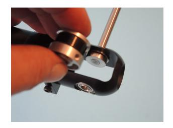
Push the tailrotor shaft thru the tailrotor housing. Note that the flat spot with the bigger distance to the end must be placed on the left side (where the grub screws of the belt wheel are).
