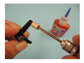
On the free end of the screw a nut D547 will be attached using Loctite.
