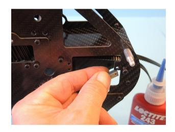
Place a frame connector D622 between the lower rear mounting holes of the roll servos and fix is provisorically on one side with a hex bolt (no Loctite).
