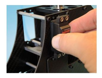
The roll servo is attached with four hex bolts M3x12 D119, washers M3 002 and lock nuts M3 008s. Therefore the open wrench #707 is a very good tool. The lower right screw will be applied with Loctite and turned then in the connector D622. After gently tightenimng of the bolts the provisorically mounted single bolt on the right side can be removed.
