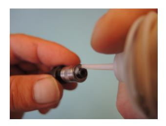
Now push the ball cage on as shown and add also a bit of lubrication on the balls.
