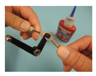
Push the first ball joint on one joint bolt and check the clearance.
