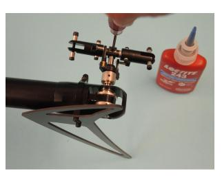
Push a hex bolt M3x16 D329 thru the bearings of the bell crank D49 and add a washer shim 3x6x1 051and apply some Loctite on the thread...
