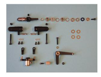
Push a conic spacer bush D256 on the tailrotor hub D255 (cone inside).
