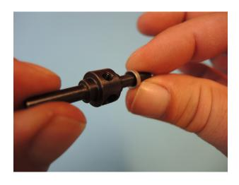
Now add a ball bearing 5x10x4 942, the blade grip holder ring 980, a washer shim 7x10x0,2 054...
