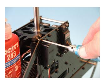
Mount the elevator servo holder D420 (attached on the elevator servo) with two hex bolts M3x6 D196.
