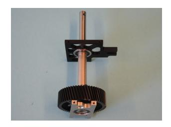
Attach the lower ball bearing block D608 on the upper right frame D602 with two hex bolts M3x6 D196 using Loctite. Tighten the bolts first if the screws of the upper mainshaft bearing block D607 are also mounted.
