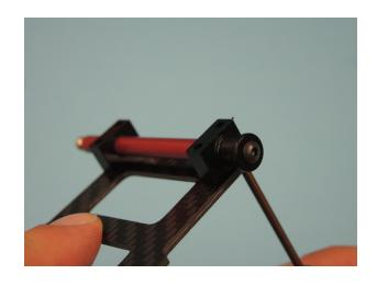
Attach the Tenax holder D460 with two hex bolts M3x12 D119 and lock nuts M3 008s on the lower right frame D625.
