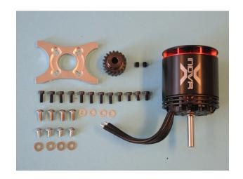
Attach the motor with for lense screws M4x8 D106 using Loctite on the motor-plate D633 so that the motor cables are placed besides. So there is more space to mount them later with the controller. For alternative motor types and bolt lengths there are M3x6 hex bolts D196, M3x8 D197, M4x6 D125 and for length reduction washer shims 3x6x1 051 and 4x8x1 043 in the bag.
