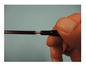
Add a pice of shrink tube on the ball joint and the carbon rod to enlarge stiffness. This side of the tail pushrod is later placed at the rear end (on the bell crank D49).
